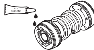
Figure 37. Applying RVT Silicone
